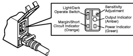
**NOTE:** The power indicator will turn off when the output indicator is on. The catalog number for the Rear Snap Cover is #60-2679.
