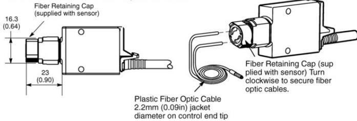
Special Glass Fiber Optic cables are also available with 2.2 mm (0.09 in) diameter control end tips.
