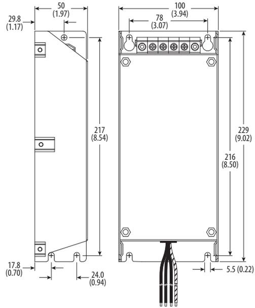
**Frame C EMC Line Filters** – Dimensions are in millimeters and (inches)
