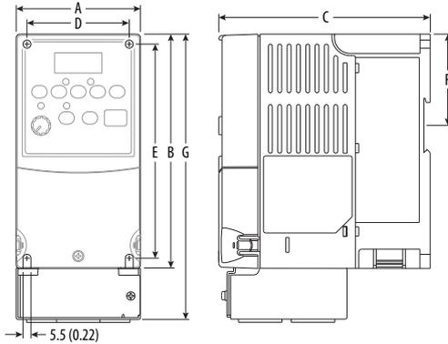
Dimensions are in millimeters and (inches). Weights are in kilograms and (pounds).
