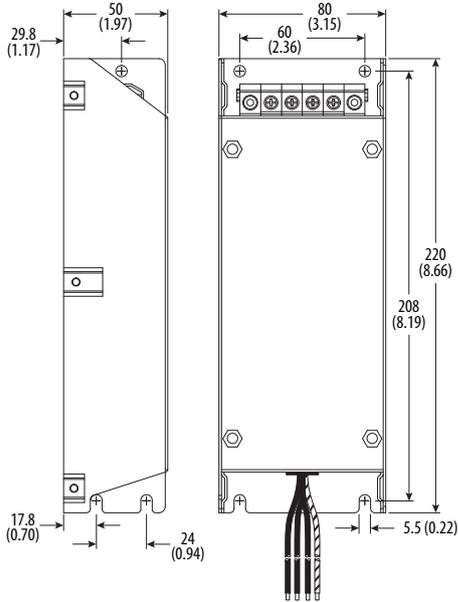
**Frame B EMC Line Filters** – Dimensions are in millimeters and (inches)
